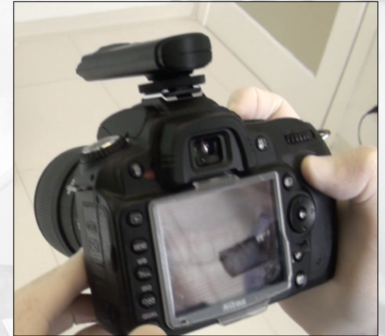
SLR camera with a commander to activate the slave flashes
