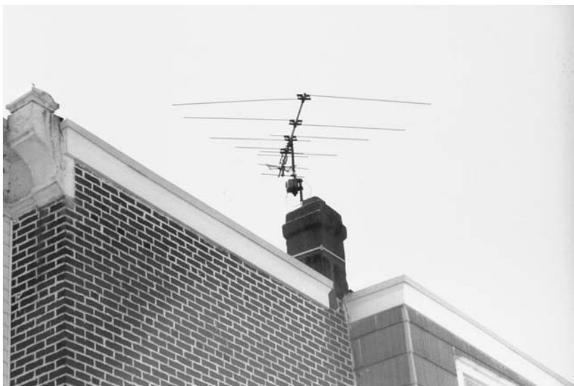
A Yagi-Uda antenna, shown here on a house in Philadelphia, is sometimes called a “television aerial.” (Kyle Kirkland)
