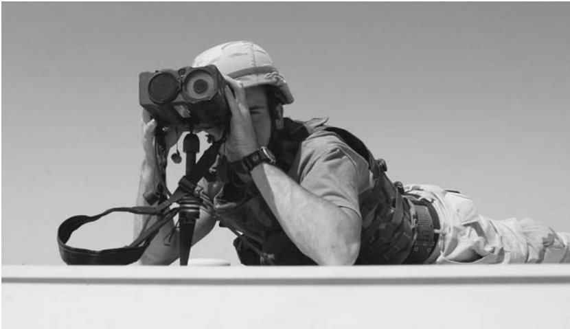
The military uses laser range finders to calculate precise distances required for pinpoint artillery and bombing missions. ( United States Air Force/Master Sgt. Robert R. Hargreaves Jr. )
