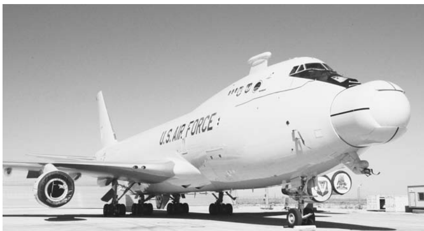
This ABL aircraft is a modified 747 carrying a powerful laser, the beam of which exits from the plane’s nose. ( Missile Defense Agency )
